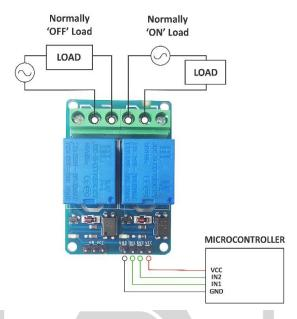
In this diagram, the relay on the left (channel 1) is connected in a regular fashion with the load and source going between common and normally open, so when the relay is activated, the load is powered. On the right channel (channel 2), the load and source are connected between common and normally closed, which means that the load is powered by default till the relay is activated.
